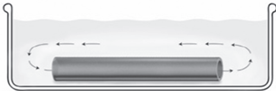
Figure 2. Practically incessant flow occurs through hydrophilic tubes immersed in water.
