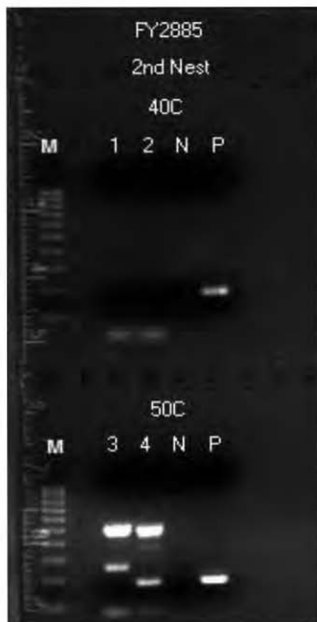
Figure 8. Detection of HPV L1 gene DNA in a postmortem splenic sample by a second same-nested PCR amplification with a non-degenerate HPV16MY11+/GP6 primer pair. Description: Four parallel same-nested PCRs with the MY11 (1)/GP6 primer pair, each started with 0.5 µg of human genomic DNA extracted from spleen, were performed, two under low stringency condition with 40°C annealing temperature and two under high stringency condition with 50°C annealing temperature. No HPV amplicon was obtained in the 1 st same-nested PCRs. Then the second same-nested PCRs each with an HPV16MY-11+/GP6 primer pair were performed. As depicted in this gel electrophoresis, an intense HPV DNA amplicon band of ~190 bp in size was generated and shown in lane 4 in one of the two second nested PCRs under high stringency condition only. However, due to co-amplification of human genomic DNA which generated a large amount of high molecular weight PCR products, it was impossible to use this material as the template for DNA sequencing.
